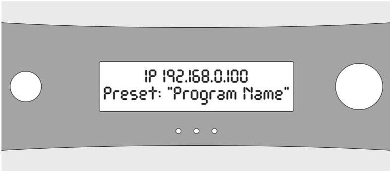
Turn the dial to select your desired preset to match your Origin Acoustics Speakers. If you are not sure which preset to use, refer to the “Amplifier Preset” section of this manual. Once you have found the desired program number it will be blinking. Press the dial to select the desired program to load, at which time it will stop blinking. If the number is not blinking while selecting, the display will return to the “Load Program” menu and you will need to restart the process.
